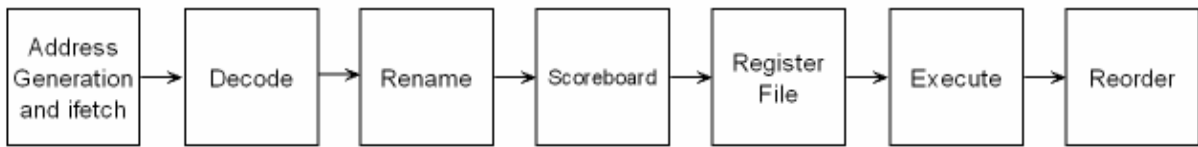
Figure 3 The processor pipeline
